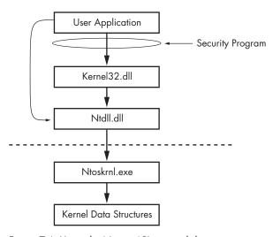
Figure 7-4: Using the Native API to avoid detection
