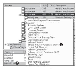
Figure 3-7L: Examining service malware in Process Explorer
