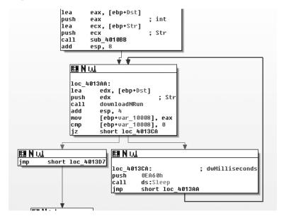
Figure 14-1L: Sleep loop with downloadNRun function
