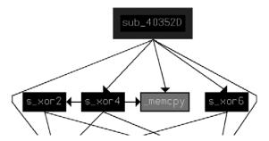
Figure 13-7L: Relationship of encryption functions
