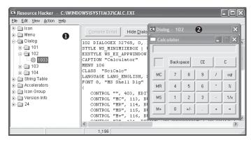
Figure 1-9: The Resource Hacker tool display for calc.exe
