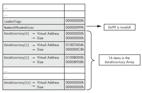
Figure 16-5: PE IMAGE\_OPTIONAL\_HEADER and NumberOfRvaAndSizes vulnerability
