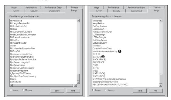
Figure 3-9L: Process Explorer shows strings that are not normally contained in sychost.exe.
