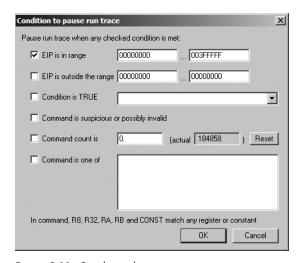
Figure 9-11: Conditional tracing
