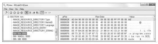
Figure 21-2L: PEview showing three different resource sections
