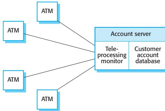
**Figure 17.9** A fat-client architecture for an ATM system
