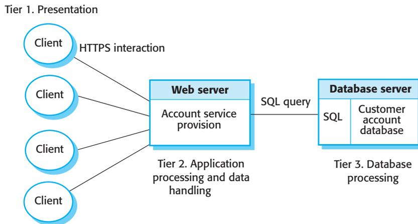
**Figure 17.10** Three-tier architecture for an Internet banking system
