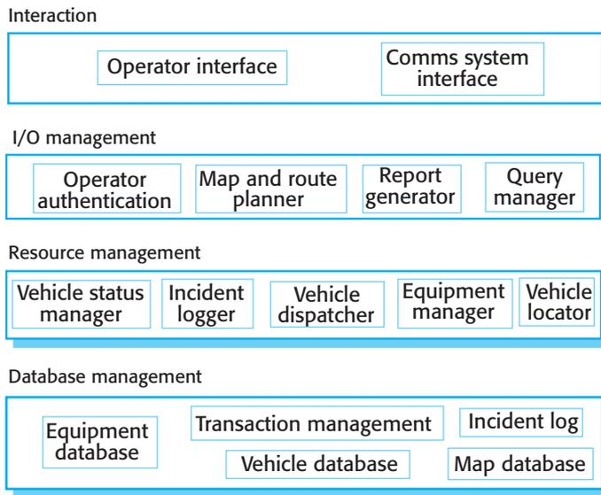
**Figure 15.9** A product-line architecture of a vehicle dispatcher system
