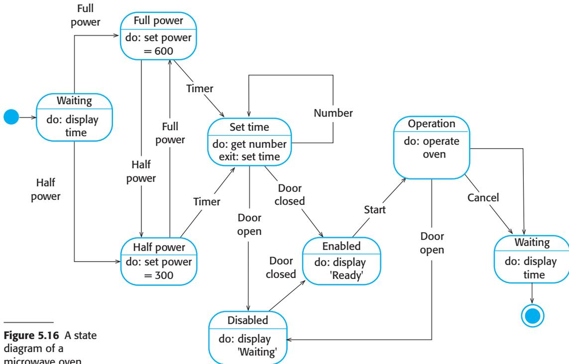
**Figure 5.16** A state diagram of a microwave oven
