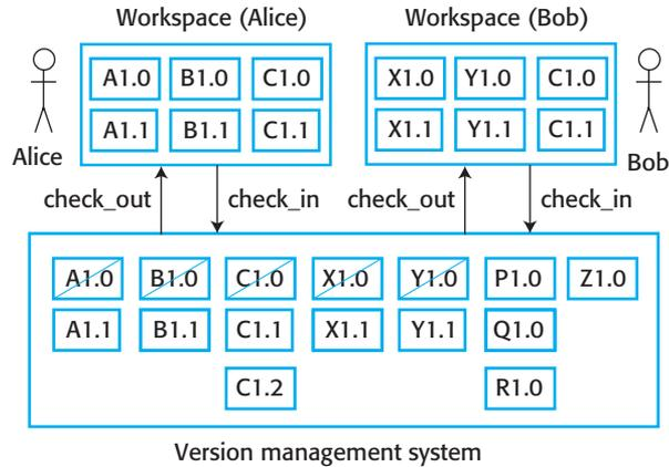
**Figure 25.5** Check-in and check-out from a centralized version repository
