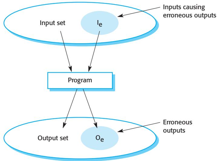
**Figure 11.2** A system as an input/output mapping
