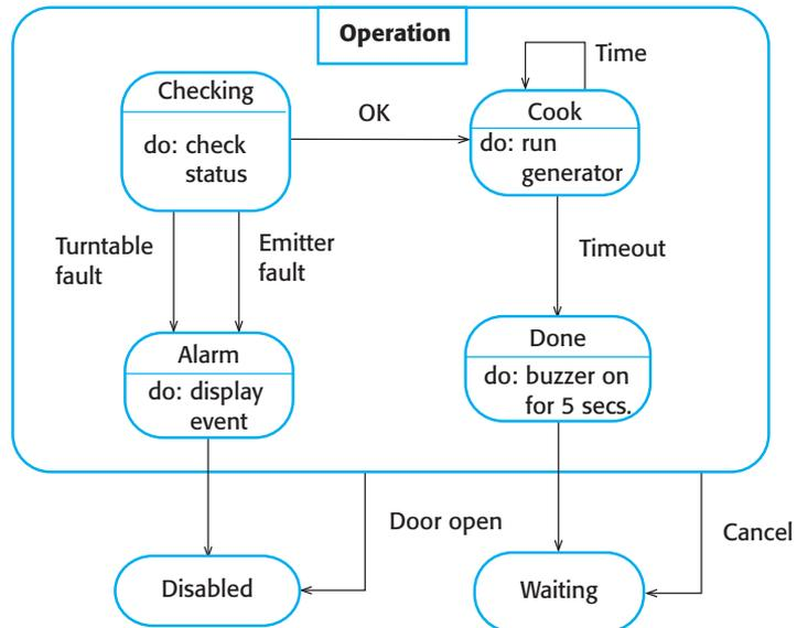
**Figure 5.17** A state model of the Operation state
