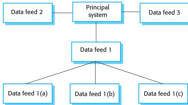
**Figure 20.11** Systems as data feeds with a unifying interface
