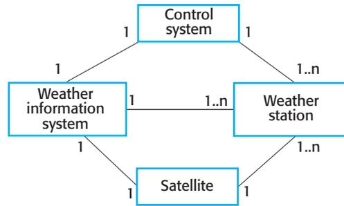
**Figure 7.1** System context for the weather station
