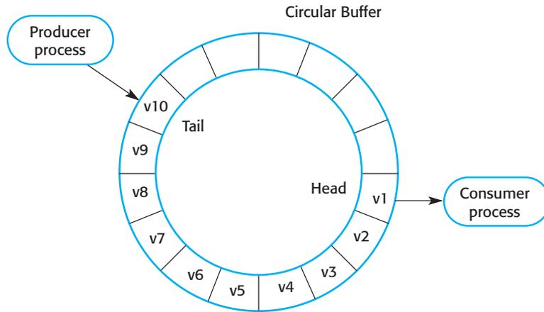
**Figure 21.4** Producer/consumer processes sharing a circular buffer
