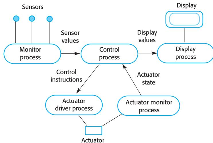
**Figure 21.10** The Environmental Control process structure
