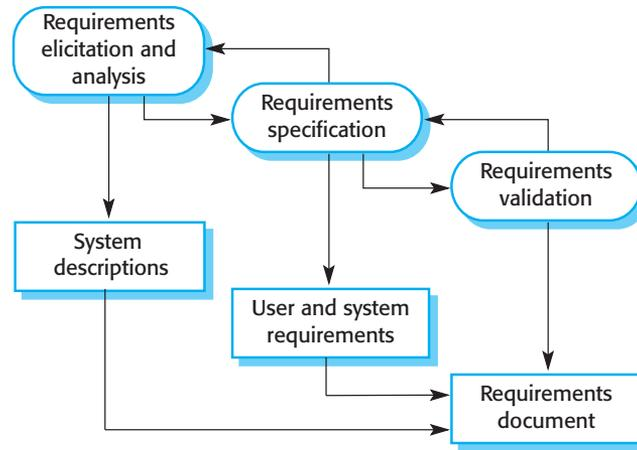
**Figure 2.4** The requirements engineering process
