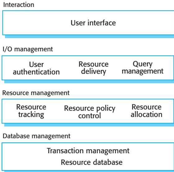
**Figure 15.8** The architecture of a resource management system
