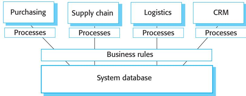
**Figure 15.13** The architecture of an ERP system
