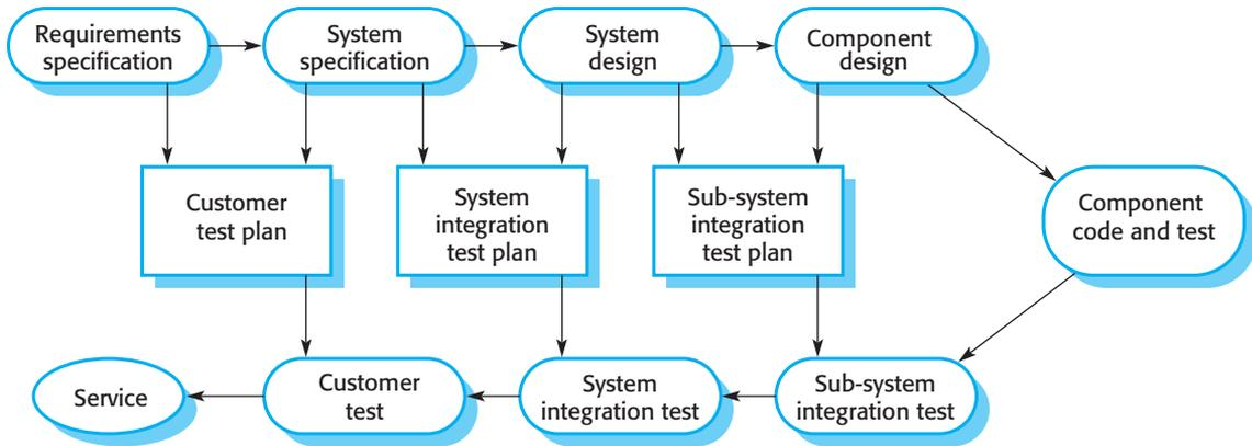
**Figure 2.7** Testing phases in a plan-driven software process
