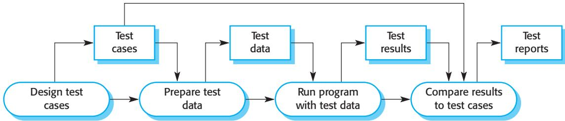
**Figure 8.3** A model of the software testing process
