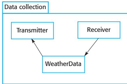
**Figure 7.5** Architecture of data collection system
