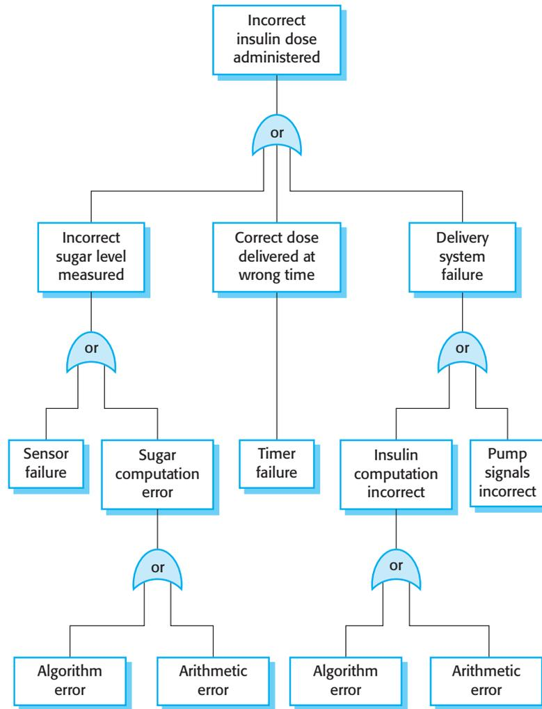
**Figure 12.5** An example of a fault tree
