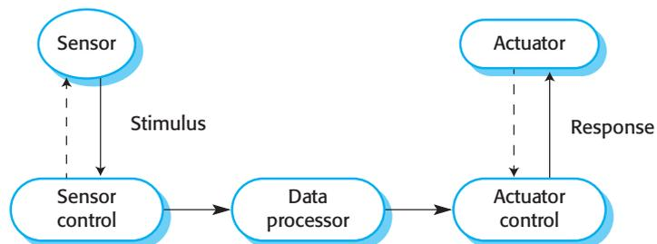
**Figure 21.3** Sensor and actuator processes
