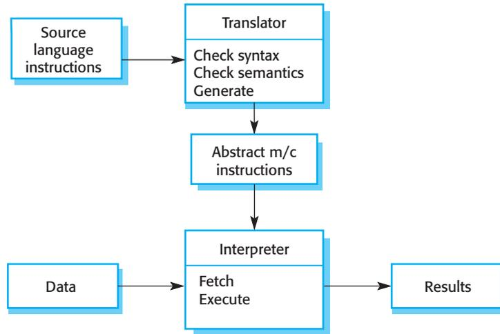
**Figure 6.20** The architecture of a language processing system
