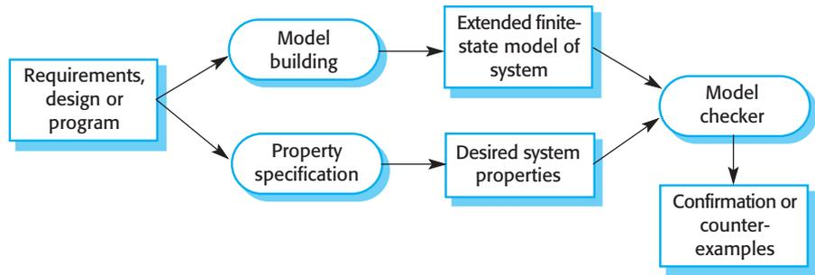
**Figure 12.8** Model checking
