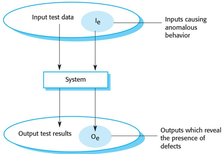
**Figure 8.1** An input-output model of program testing
