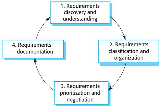
**Figure 4.7** The requirements elicitation and analysis process
