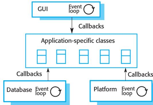
**Figure 15.6** Inversion of control in frameworks
