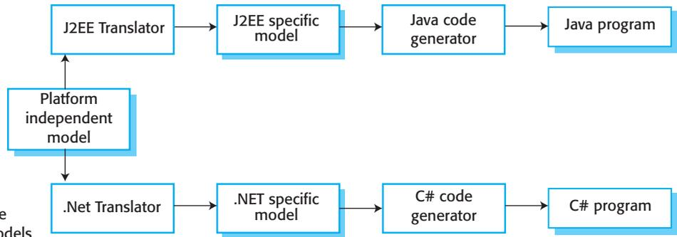
**Figure 5.20** Multiple platform-specific models
