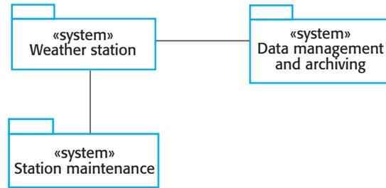
**Figure 1.7** The weather station's environment
