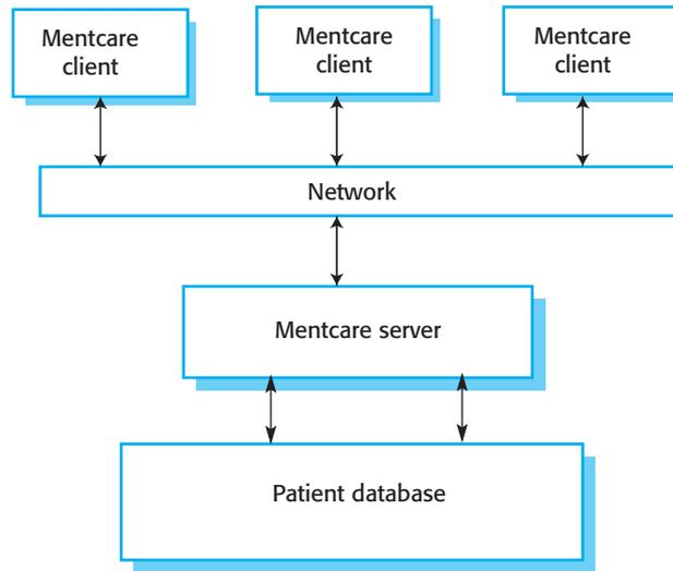
**Figure 14.10** The client–server architecture of the Mentcare system
