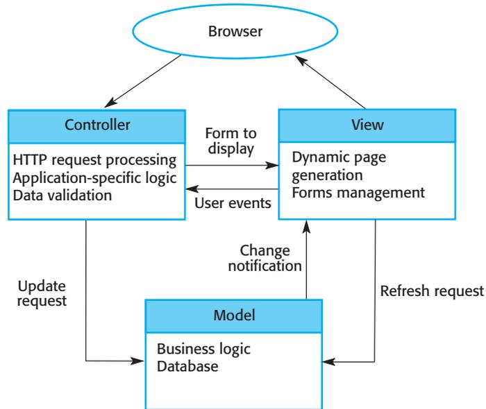
**Figure 6.6** Web application architecture using the MVC pattern
