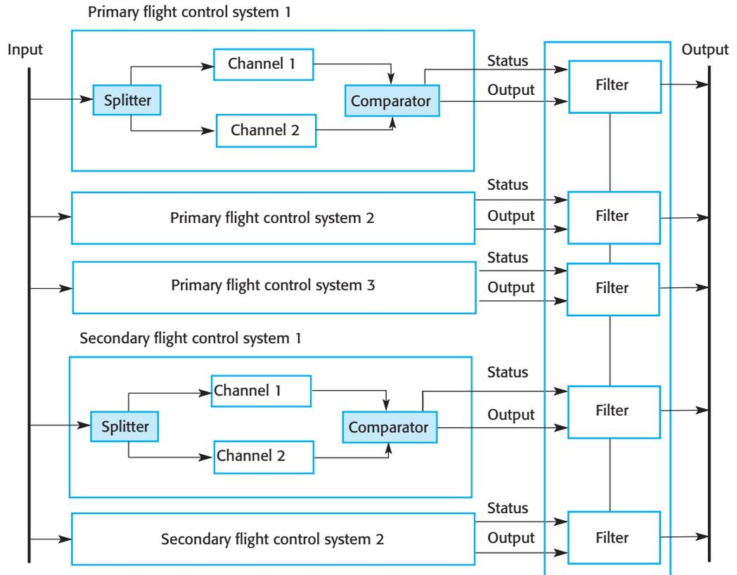
**Figure 11.8** The Airbus flight control system architecture
