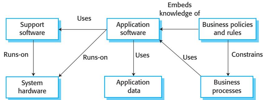
**Figure 9.7** The elements of a legacy system
