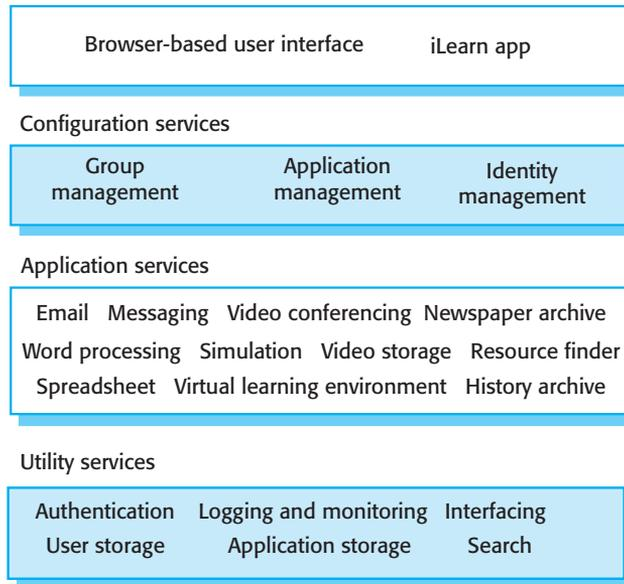
**Figure 1.8** The architecture of a digital learning environment (iLearn)
