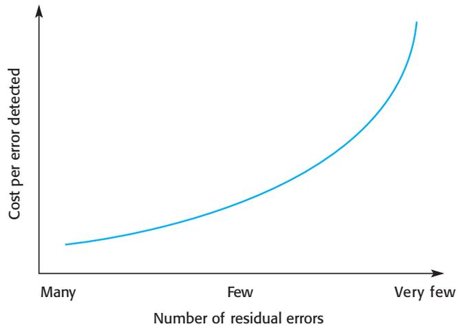
**Figure 11.1** The increasing costs of residual fault removal
