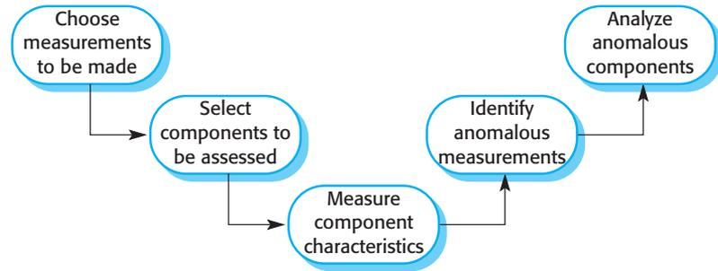
**Figure 24.13** The process of product measurement
