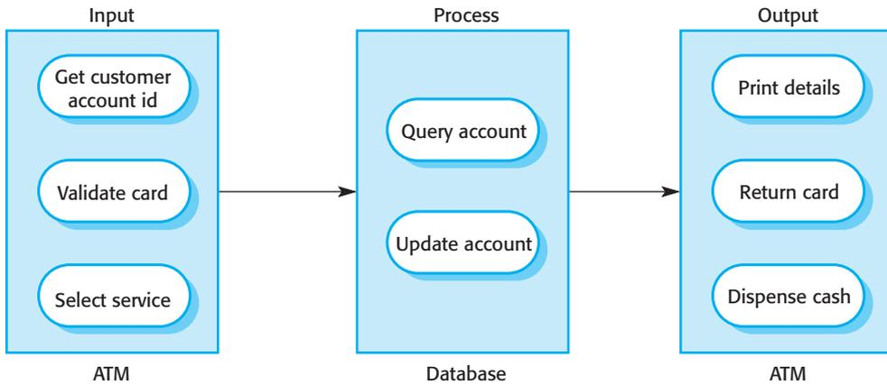
**Figure 6.17** The software architecture of an ATM system
