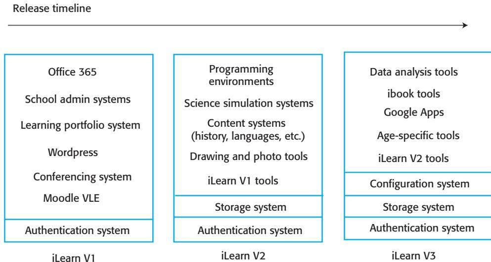
**Figure 20.8** Release sequence For the iLearn SoS
