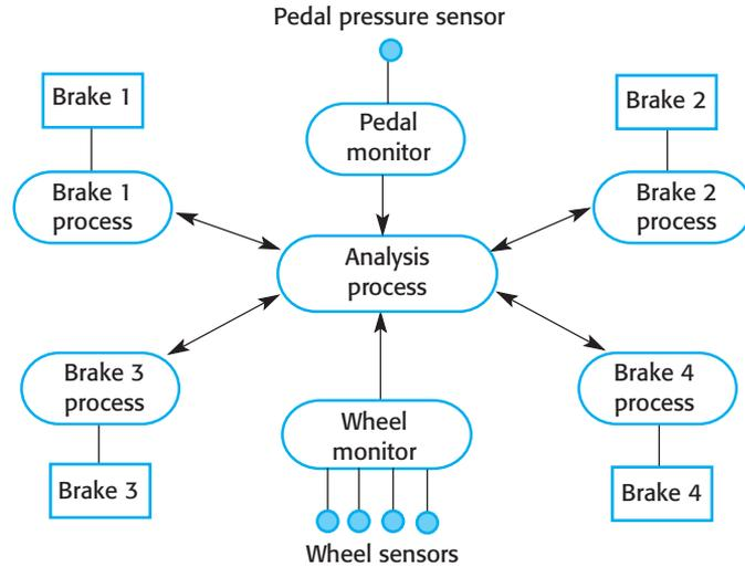
**Figure 21.11** Control system architecture for an anti-skid braking system
