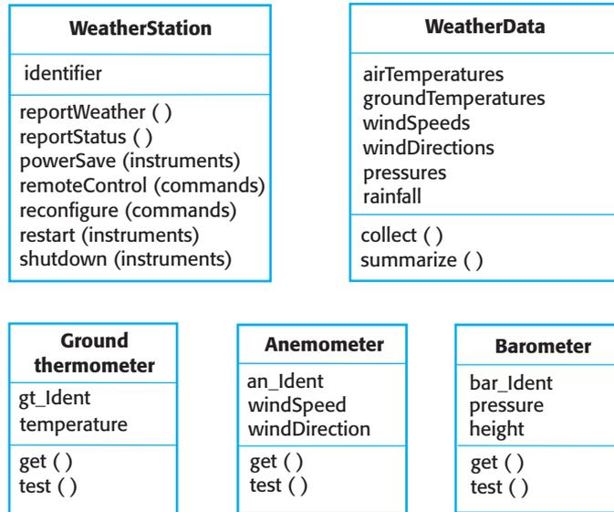
**Figure 7.6** Weather station objects
