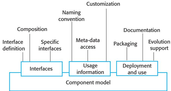
**Figure 16.4** Basic elements of a component model
