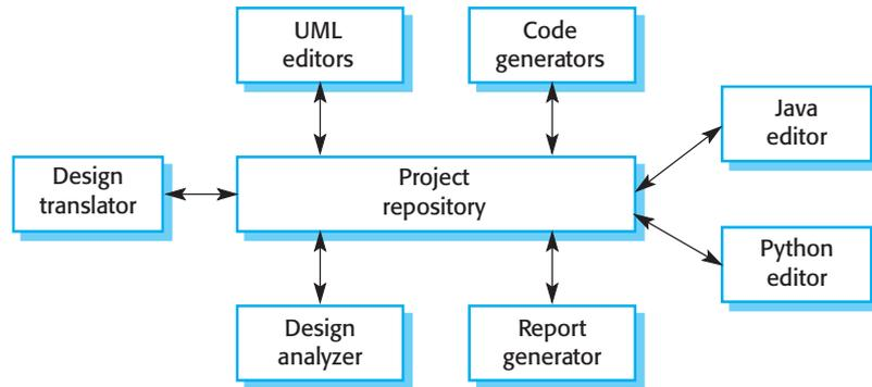
**Figure 6.11** A repository architecture for an IDE
