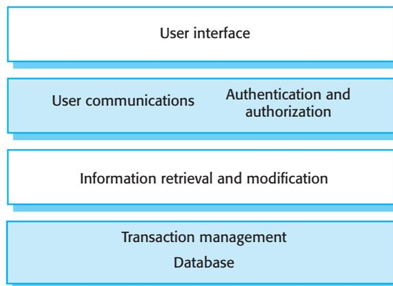
**Figure 6.18** Layered information system architecture
