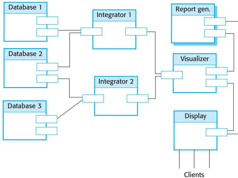
**Figure 17.13** A distributed component architecture for a data-mining system
