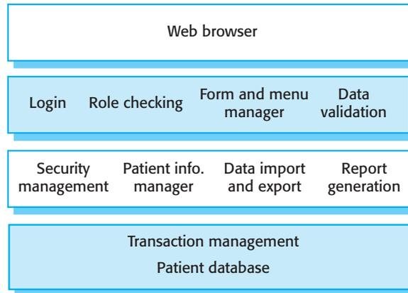
**Figure 6.19** The architecture of the Mentcare system
