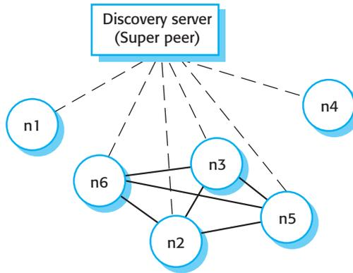
**Figure 17.15** A semicentralized p2p architecture
