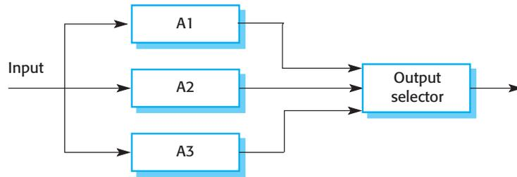
**Figure 11.9** Triple modular redundancy
