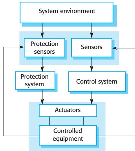
**Figure 11.6** Protection system architecture
