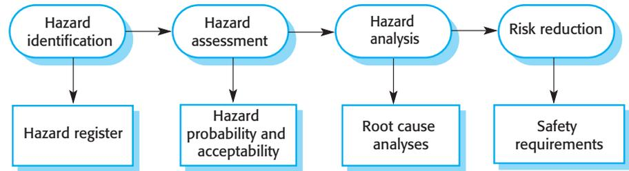
**Figure 12.2** Hazard-driven requirements specification
