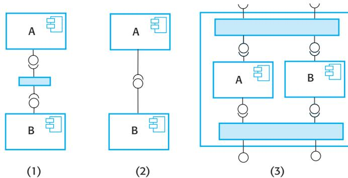
**Figure 16.10** Types of component composition
