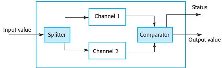
**Figure 11.7** Self-monitoring architecture
