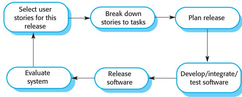
**Figure 3.3** The XP release cycle
