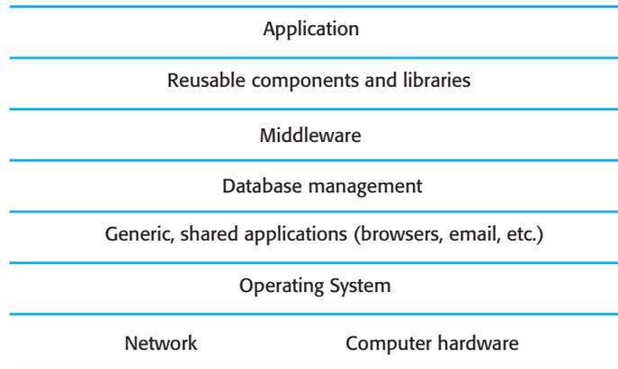
**Figure 13.1** System layers where security may be compromised
