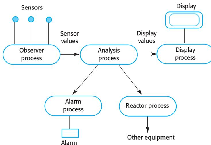
**Figure 21.7** The Observe and React process structure
