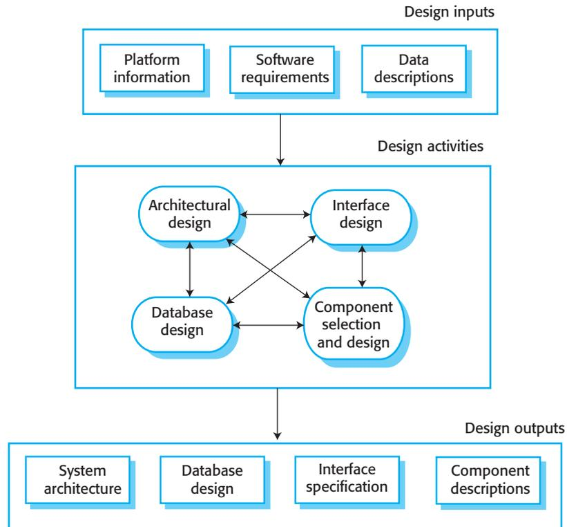
**Figure 2.5** A general model of the design process
